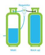
When the main bottle is empty, the regulator changes over to the back up bottle and the indicator turns red.
